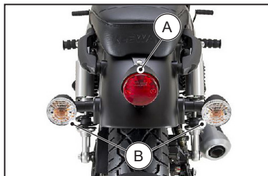
A. Brake/tail light B. Turn signal lights
