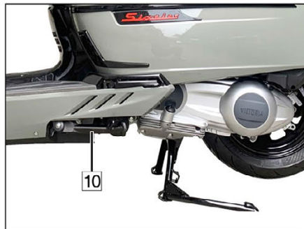
7. Side (10) switch at horizontal position.
